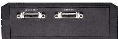
Smart Reader M4 with extension - Camera Link connectors
