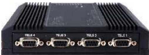
Smart Reader M5 standard - Camera LVDS connectors
