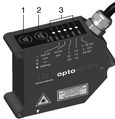
Fig. 4 Keys and LED's on the sensor
