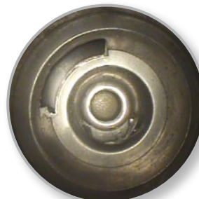
Checking brake cylinder for burrs
