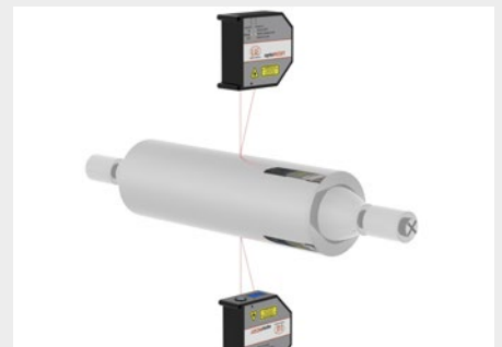
Testing the radial run out of rollers
